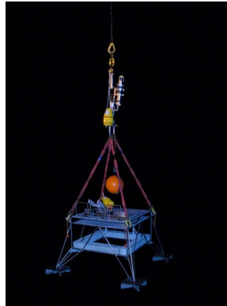
Figure 12. Anode assembly during deployment
