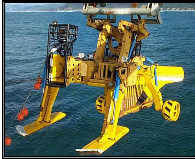
Figure 2-19 Example of a Submarine Cable Plow
