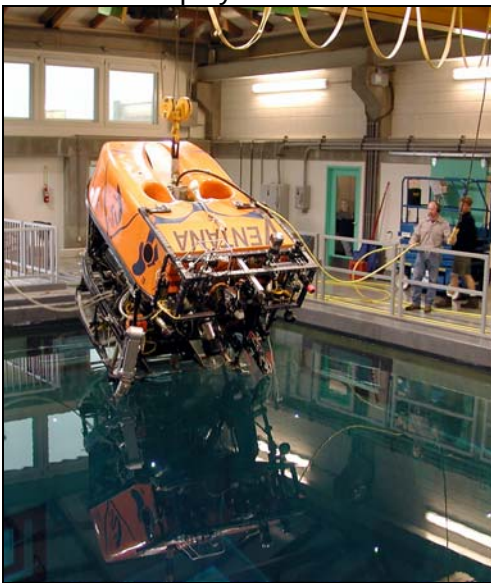
Figure 1: the ROV Ventana being lowered into the test tank
