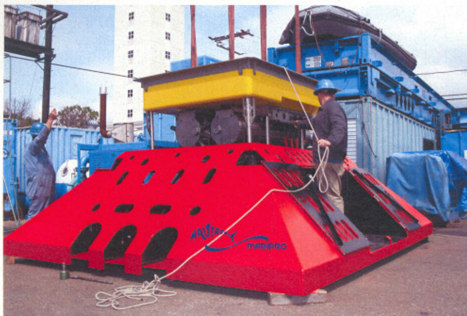
MARS science node (yellow) being placed in trawl resistant frame (orange).
