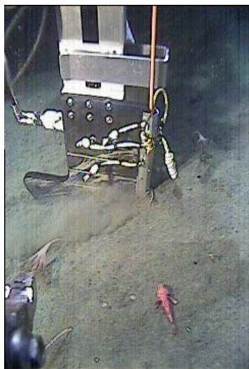
The cable laying tool sled plow
