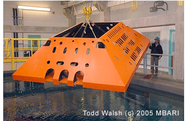
Fig. 4. MARS node trawl-proof cage undergoing tank testing prior to deployment.
