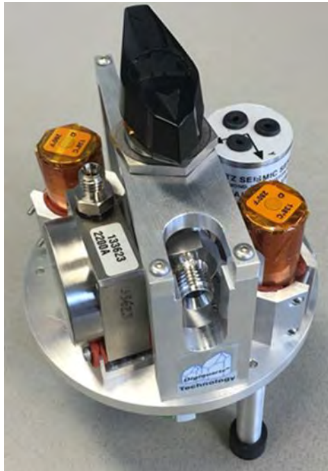
Figure 1. Prototype of the GODS (Geodesy Ocean Disaster Sensor), which is inside the GSSM housing. For cabled deployments, this is combined with an actuator to turn the valve and electronics to acquire data and interface to the cable.
