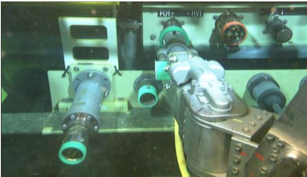
Figure 2. ROV manipulator arm being used to connect a cable to the MARS node.
