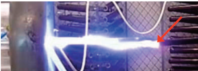
Fig. 10. CUT#5. Photo of flashover.
