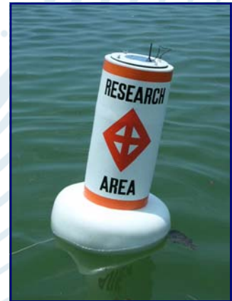
CUB-1 buoy - Sends real time data to PC's and cell phones about fish detection by the SUR below!
