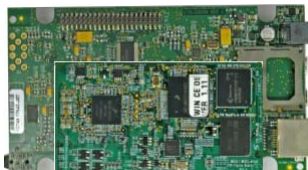
Figure 3.5 Install CPU Board onto Personality Board
