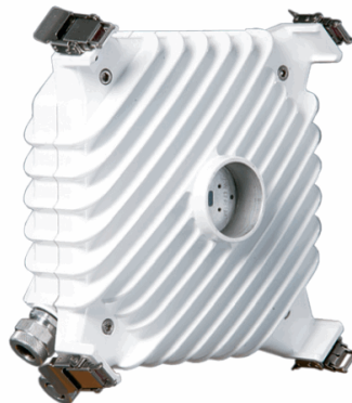
Figure 1 ExtendAir (FDD) digital microwave radio shown without antenna
