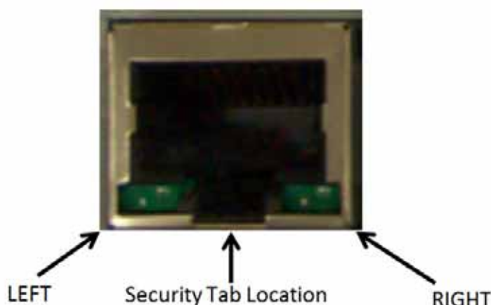
Figure 7 RJ-45 LED orientation
