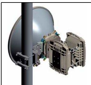
Figure 3-8: RFUs in 1+1, 2+0 or F/D Outdoor with RF Combiner
