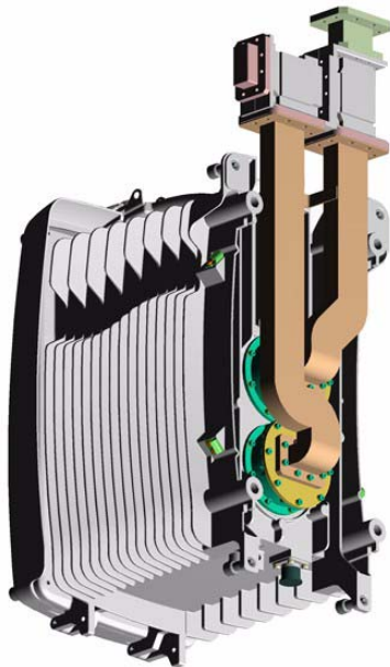
Figure 2-7: A Protected RFU, Frequency Diversity
