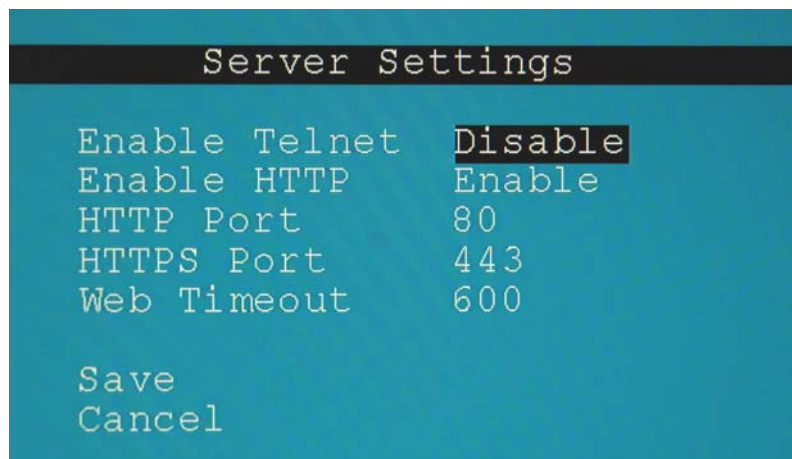
Figure 65- OSD Server Settings
