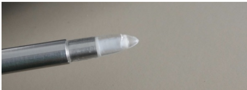
Figure 38: A shear probe with a crack in the silicone tip.
