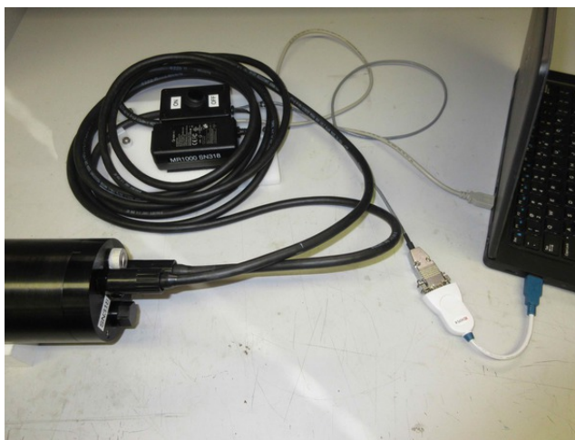
Figure 32: Connecting the deck cable to the computer.
