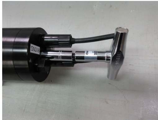
Figure 16: Removing the sealing nut.
