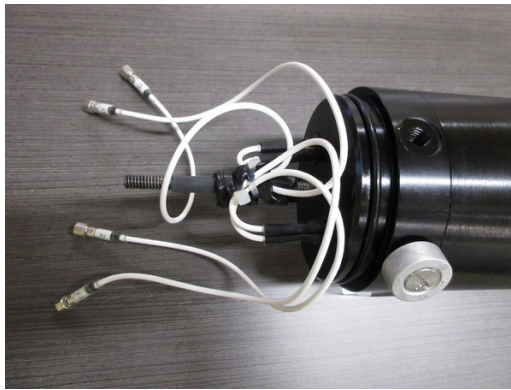
Figure 23: Nose cone removed, revealing the SMC cables and the threaded rod.
