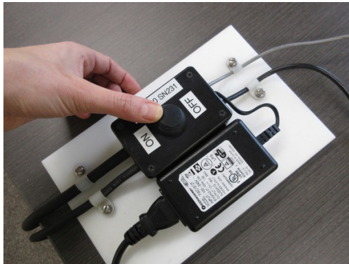
Figure 30: Sending the ON signal using the deck unit switch.
