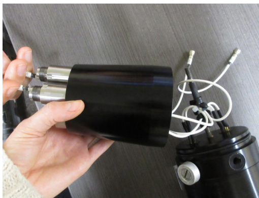
Figure 26: Feeding the SMC cables through the nose cone
