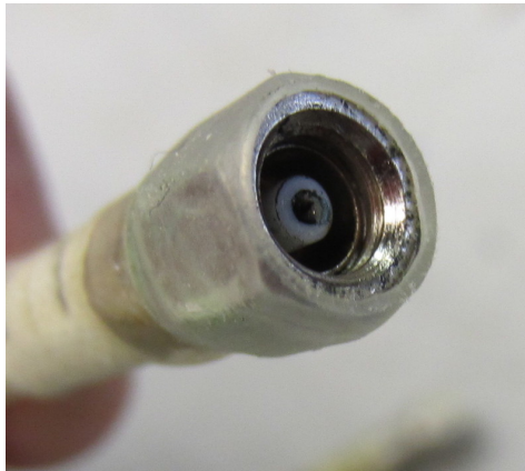
Figure 36: Green corrosion on the inside pin of an SMC connector. Without corrosion, the pin would appear shiny and gold.
