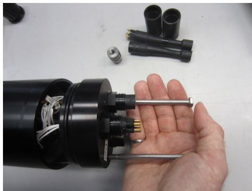
Figure 17: Leverage to Remove the Rear Bulkhead
