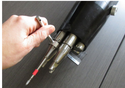
Figure 13: Tightening the probe holder.
