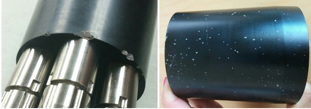
Figure 35: Extreme corrosion on a MicroRider1000 after a long-term deployment
