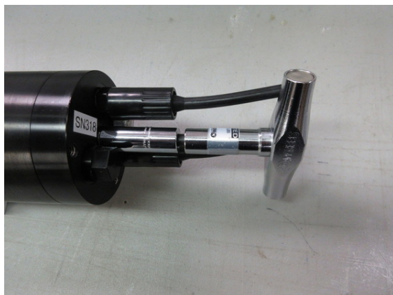
Figure 29: Tightening the sealing nut on the rear bulkhead.
