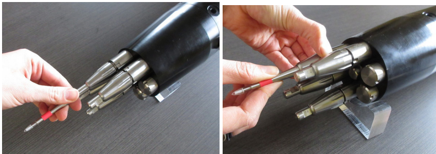
Figure 12: Inserting a probe into a probe holder.
