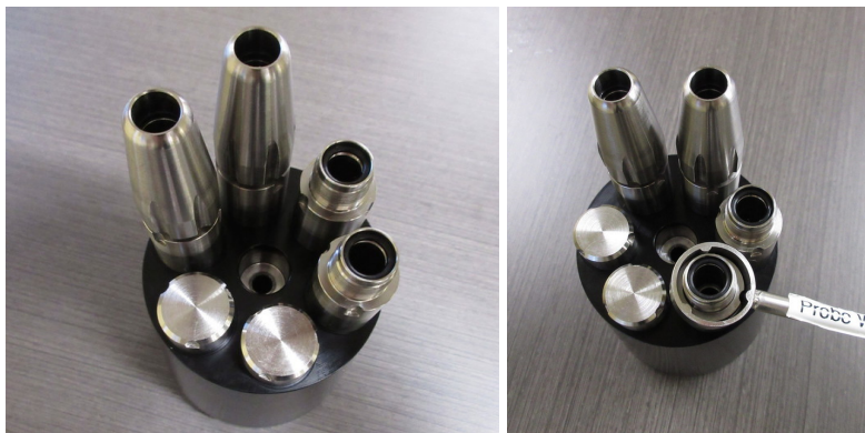
Figure 24: Removal of the probe holders from the nose cone.
