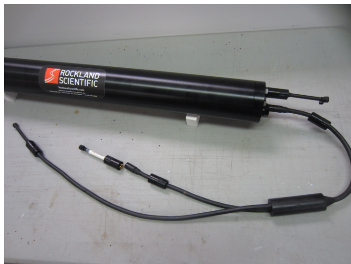
Figure 44: MicroRider-1000 with WireWalker and RBRfermata battery connection cable. The shorting ON plug is shown about to be inserted into the 8-pin connector on the cable.
