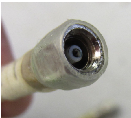
Figure 42: Green corrosion on the inside pin of an SMC connector. Without corrosion, the pin would appear shiny and gold.
