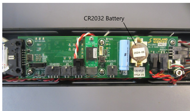
Figure 8: CR2032 Battery on Rockland Data Logger board
