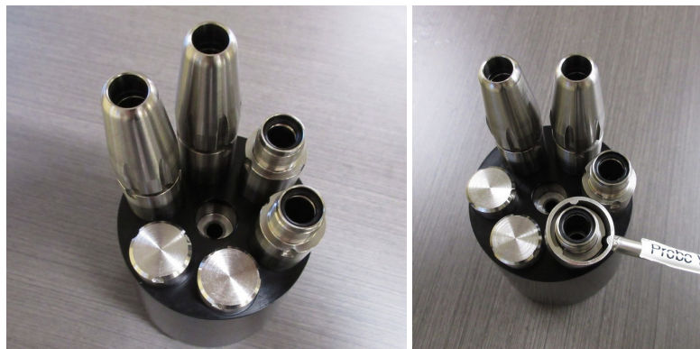
Figure 24: Removal of the probe holders from the nose cone. Note: AEMG-1 G sensor not shown.
