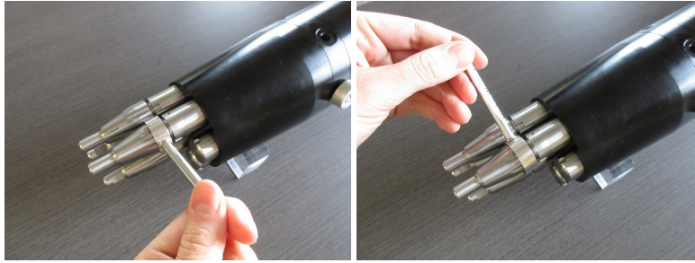
Figure 10: Loosening the probe holder using the custom probe wrench.
