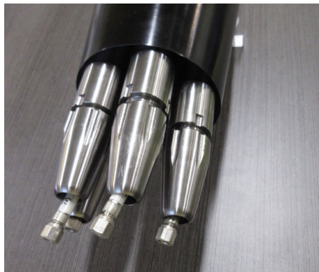
Figure 21: Nose cone after removal of test probes.
