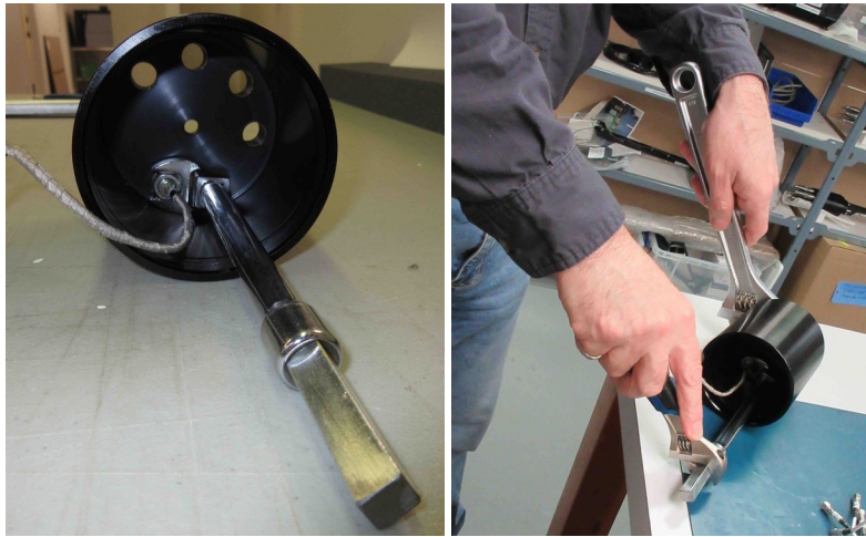
Figure 25: Using the crowfoot wrench on AEM1-G retaining nut to remove the sensor from the nose cone.
