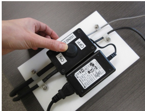
Figure 32: Sending the ON signal using the deck unit switch.
