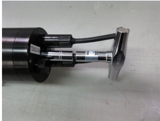
Figure 31: Tightening the sealing nut on the rear bulkhead.
