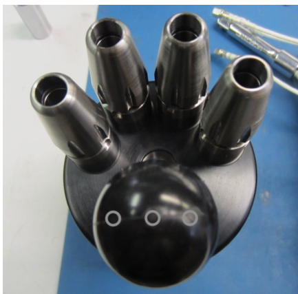
Figure 26: Alignment of the AEM1-G sensor on the nose cone. The grey circles have been enhanced for clarity.
