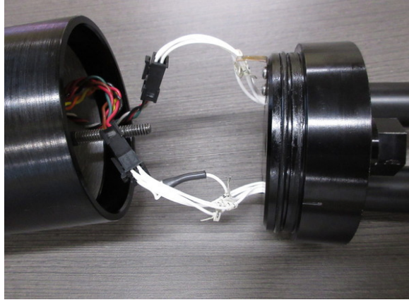
Figure 18: Disconnecting the rear bulkhead connections
