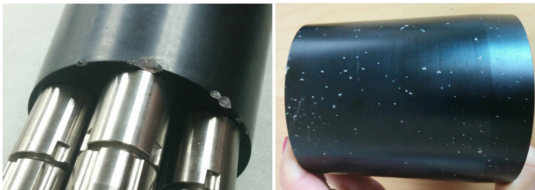
Figure 41: Extreme corrosion on a MicroRider1000 after a long-term deployment
