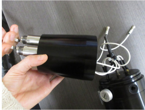
Figure 27: Feeding the SMC cables through the nose cone. The picture shows the probe holders already installed on the nose cone. It is recommended that you first install the nose cone, and then install the probe holders. Note: The instrument pictured does not have an AEM1-G EM sensor.
