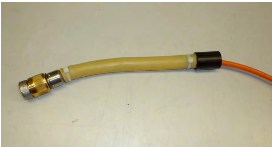
Figure 16: Latex tube installed and seated.
