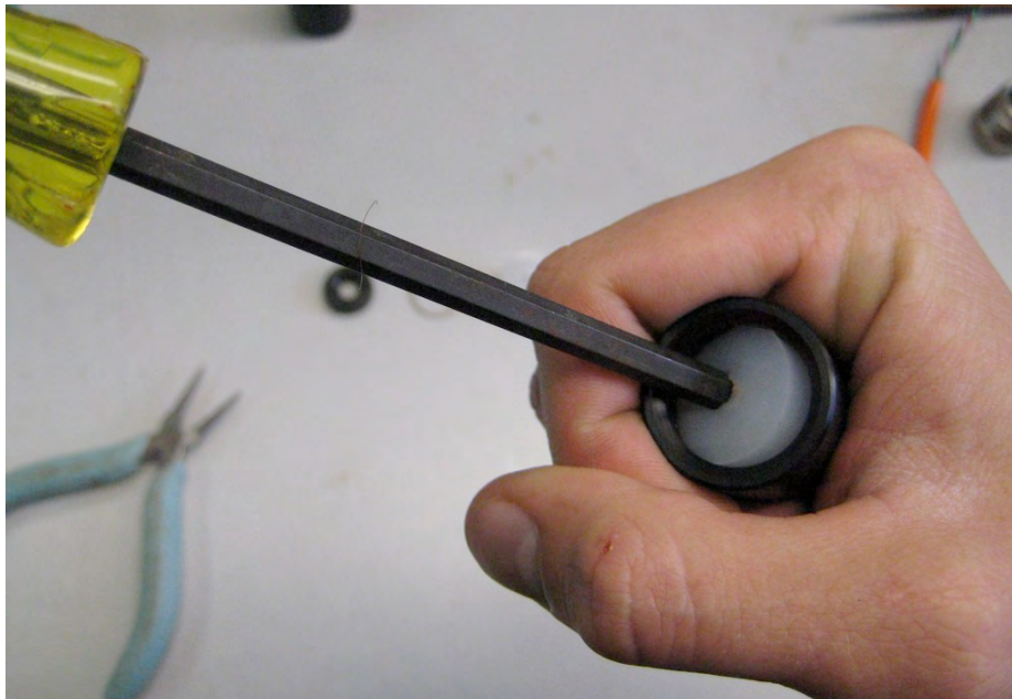
Figure 7: Removing Morrison seal.
