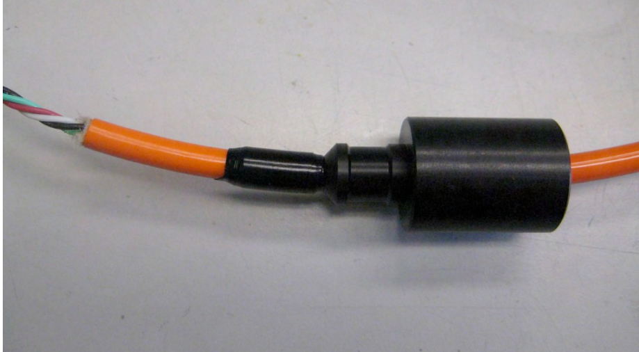
Figure 13: Electrical tape applied as a stop for the Morrison seal assembly.
