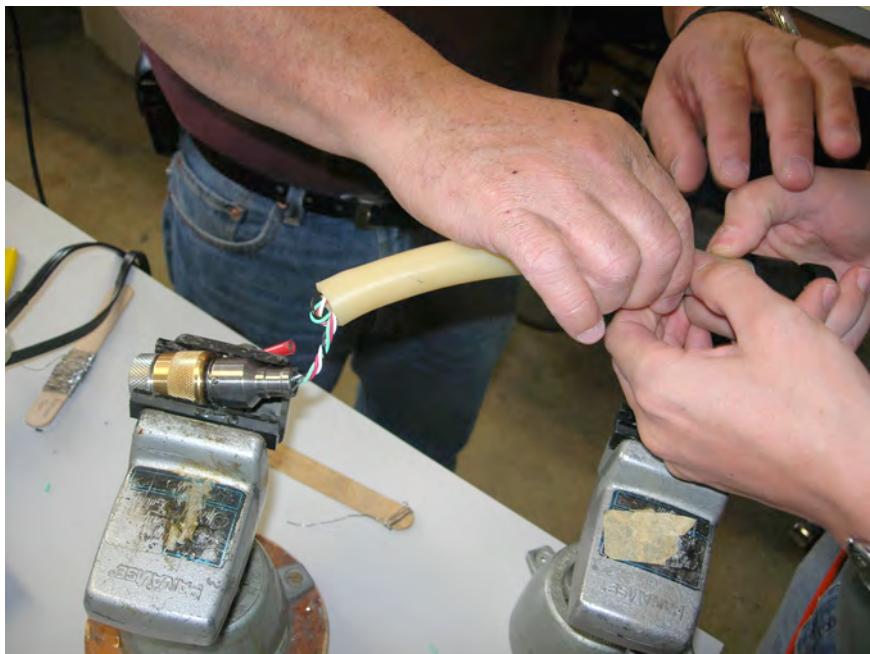
Figure 12: Latex tube installation.
