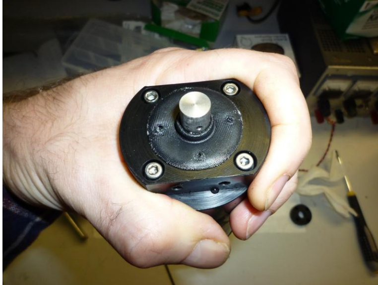
Figure 3: Front retainer removed and diaphragm mounting holes aligned with housing.
