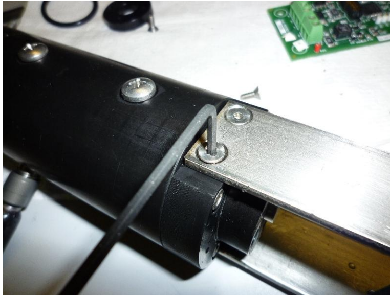
Figure 1: Removing the lever plate assembly.
