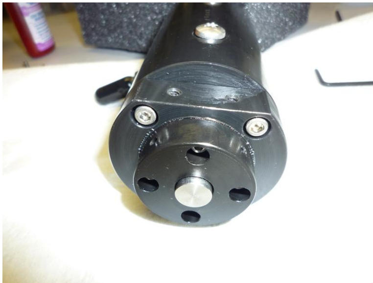
Figure 4: New Front Retainer installed.
