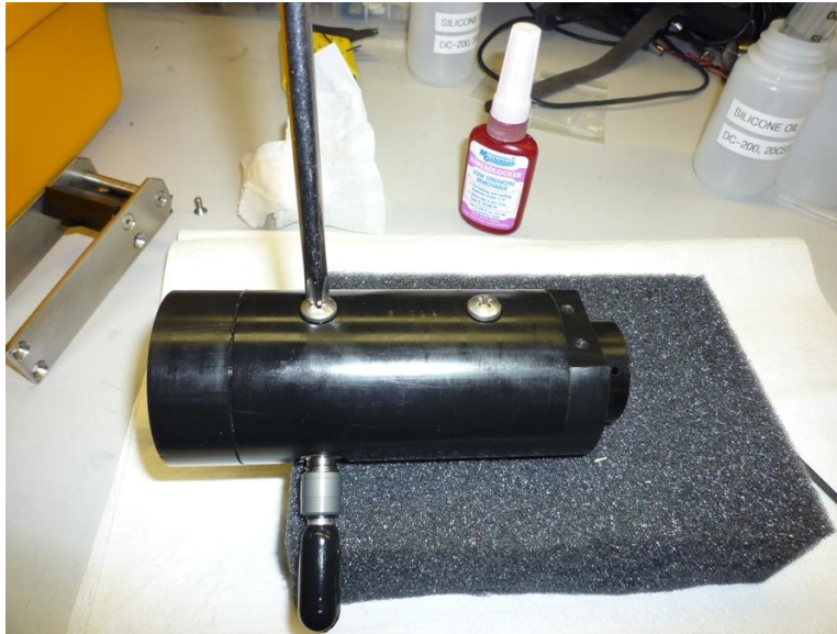
Figure 5: Removing aft sealing screw.
