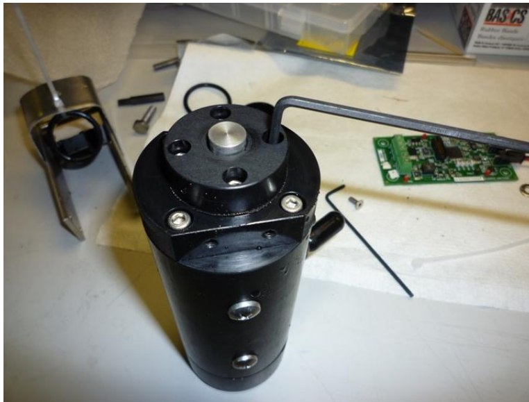
Figure 2: Removing the front diaphragm retainer.
