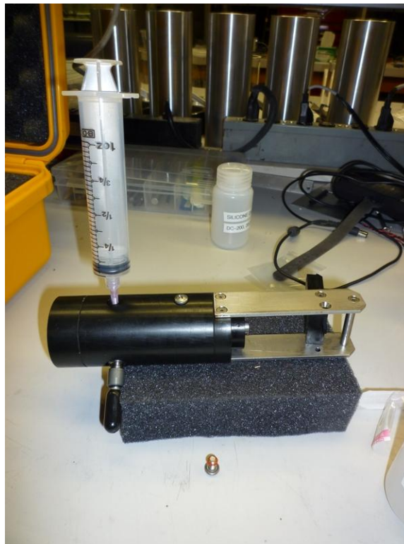
Figure 6: Inserting syringe and needle into housing.
