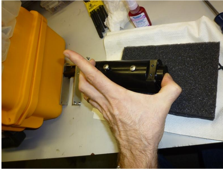
Figure 9: Making sure the rear diaphragm is slightly compressed and the solenoid plunger is fully retracted whilst installing the aft sealing screw.
