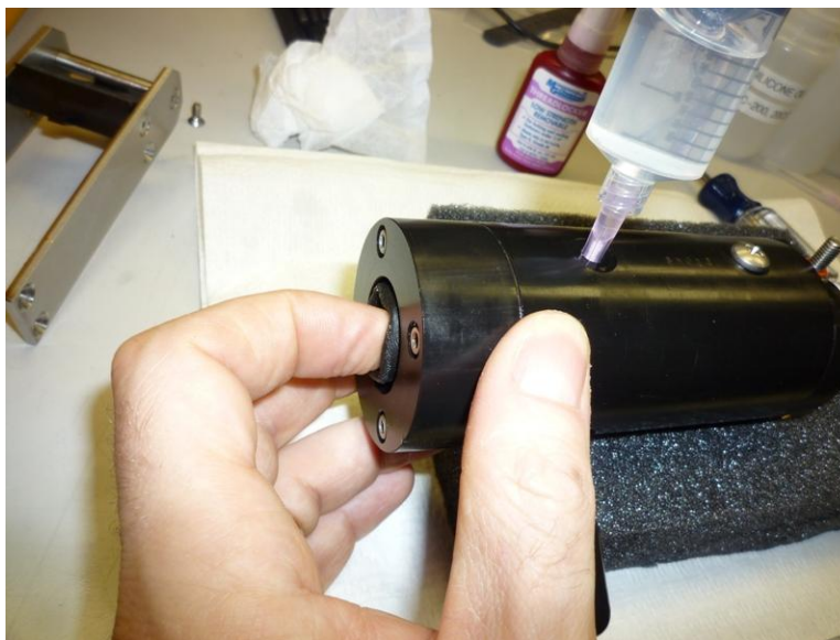
Figure 8: Injecting oil while slightly compressing the rear diaphragm.
