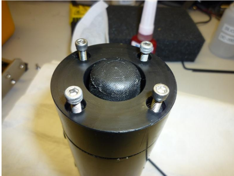
Figure 7: Rear diaphragm uncompressed - note the retaining screws are not fully seated.
