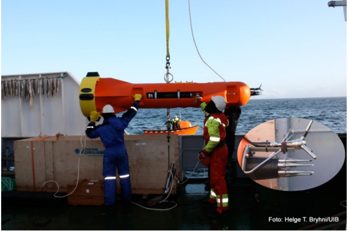
Figure 26: A turbulence measuring mooring being deployed. It carries shear probes, thermistors, and a Vector current meter (oval insert, lower right side). A nine-component motion package is inside of the pressure case. Photo courtesy of Helge Bryhni, University of Bergen.
