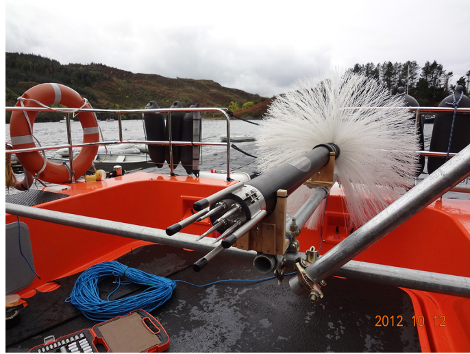
Figure 3: The VMP-200 mounted into its deck holder with the sensors facing the camera. The four prongs are guards protecting the two shear probes and thermistors mounted on to the bottom end of the profiler. The drag brushes are the white plumage at the top end. The tether-line is the blue cordage laying on deck.
