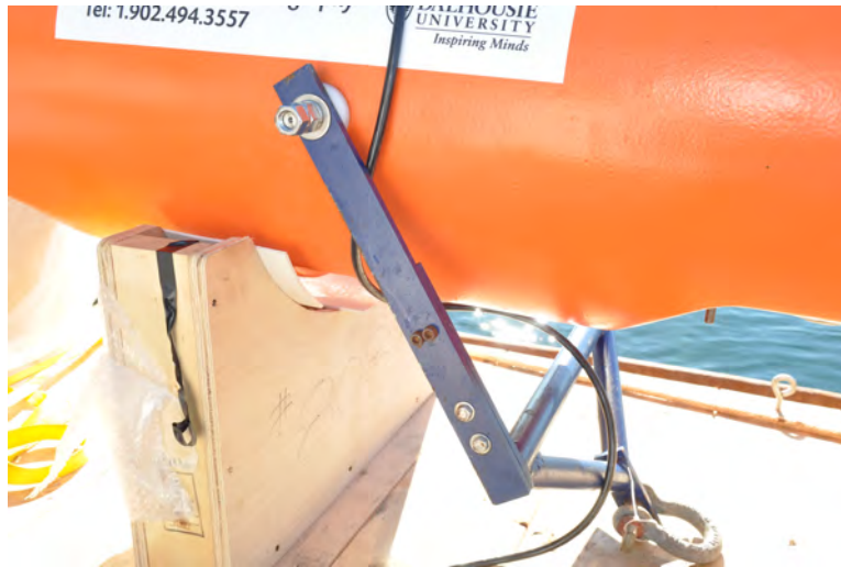
Figure 3: A close up view of the bridle. During slack water the Nemo pitches up until it is arrested by the horizontal member of the bridle.
