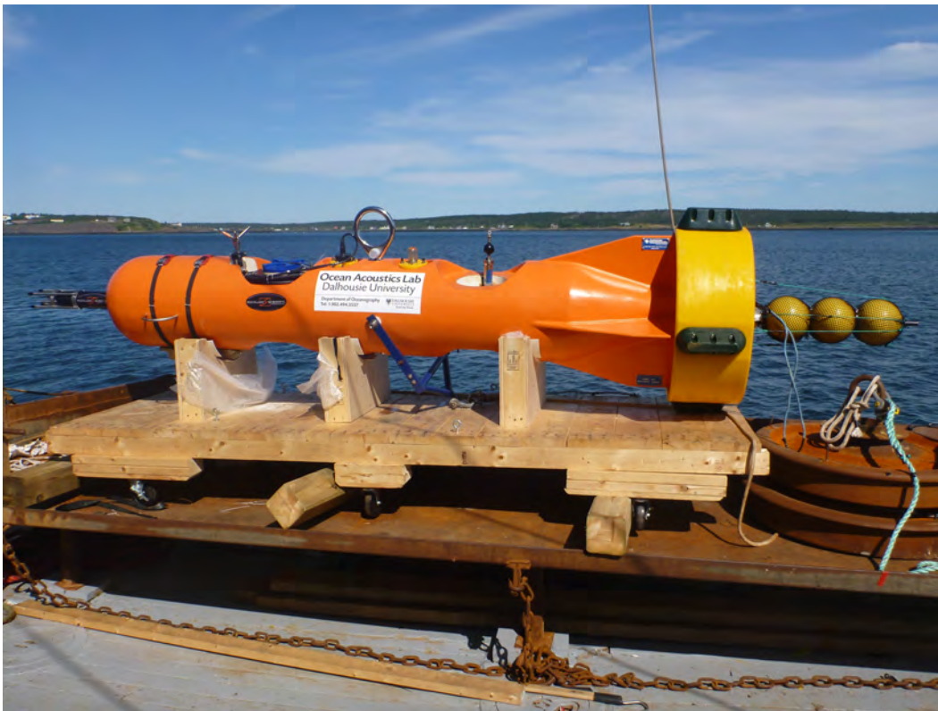
Figure 1: The Nemo shortly before its deployment in Grand Passage. The black pressure case protruding from the nose is the MicroRider turbulence measurement system. The Vector CM is just aft of the two straps used to tie lead weight to the underside of the float. Extra floatation was added aft of the tail fin. The yoke for the anchor line is the blue structure near mid body.
