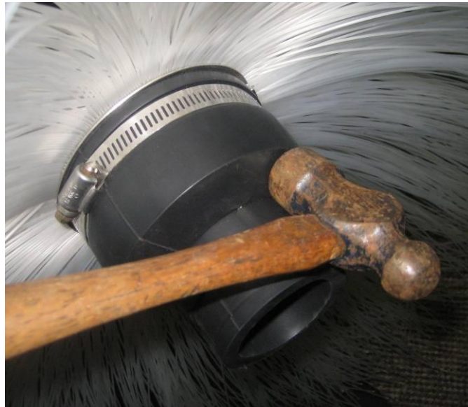
Figure 13: Tightening brushes to tail section.
