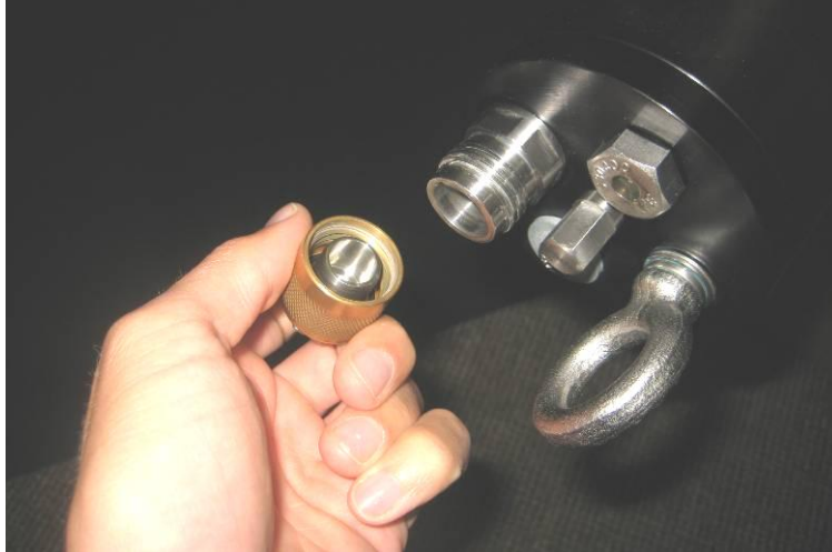
Figure 2: Removing the MHDG cap from the MHDG bulkhead connector on the VMP-200-IR rear bulkhead. This connector pair has two o-rings; the female cap (in left hand) has an o-ring that falls out easily during handling.
