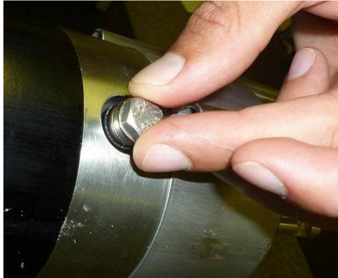
Figure 9: Attaching magnet to front bulkhead to turn on instrument.
