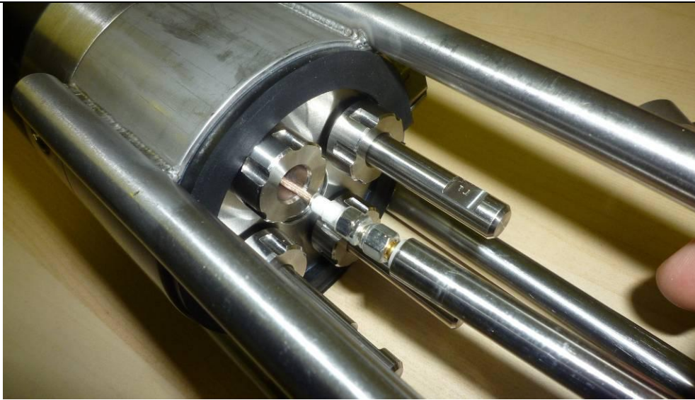
Figure 18: Removing Dummy Probe. Note the clear heat shrink tubing around the SMC connector.
