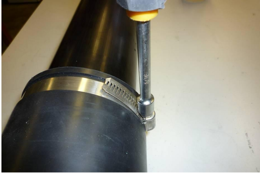
Figure 16: Attaching tail section to pressure case using straight rubber coupler.
