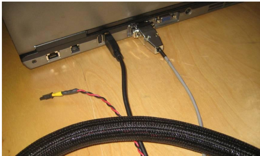
Figure 6: Connecting the USB cable from the UTRANS to your computer. The COM port (gray cable) is not normally used with a VMP-200-RT.
