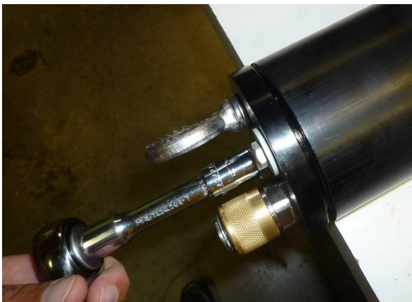
Figure 24: Tightening the sealing nut.
