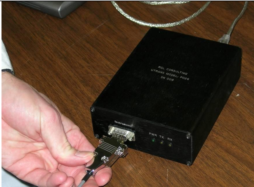
Figure 5: Connecting Deck Cable 9-pin D-sub connector to the UTRANS. Note that this is a proprietary high-speed link and not a standard RS-232 COM connector.
