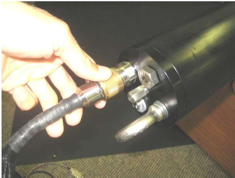
Figure 3: Connecting the deck cable to the VMP-200-IR rear bulkhead.
