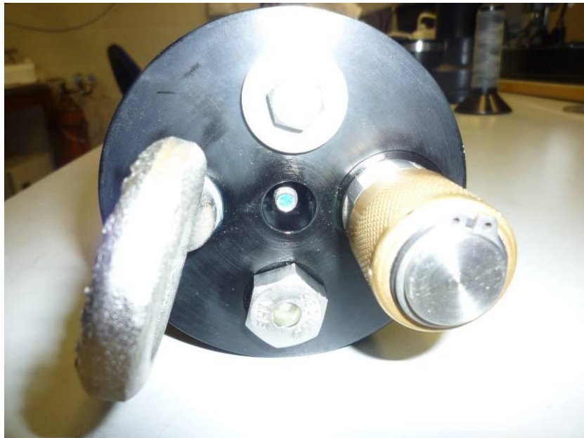
Figure 23: Rear bulkhead inserted onto end of tube with threaded rod extending through the bore.
