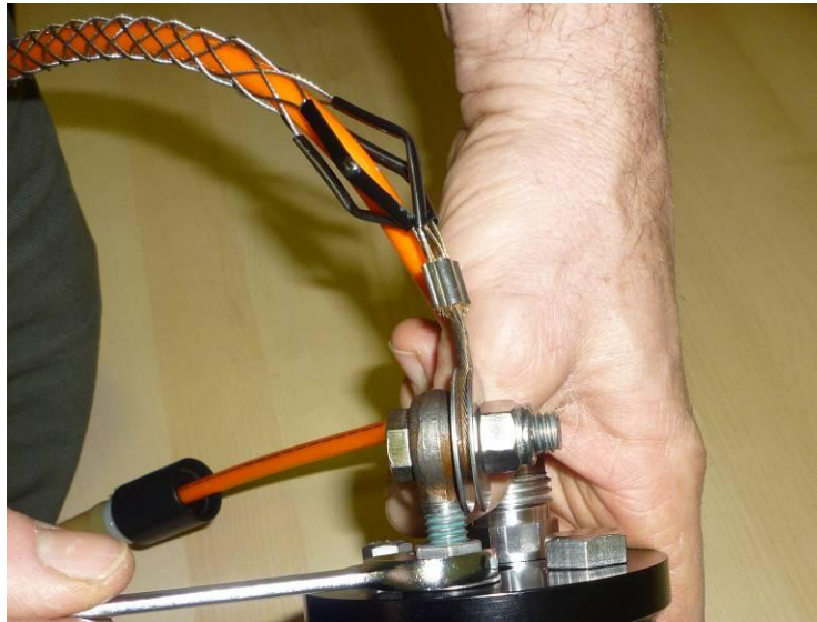
Figure 15: Attaching underwater cable tether to VMP-200-RT.
