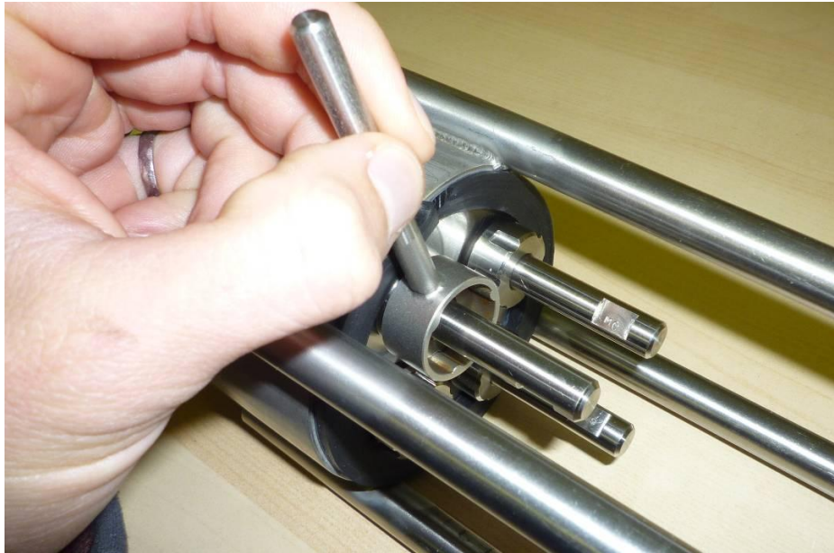
Figure 17: Loosening the probe holder using custom probe wrench.
