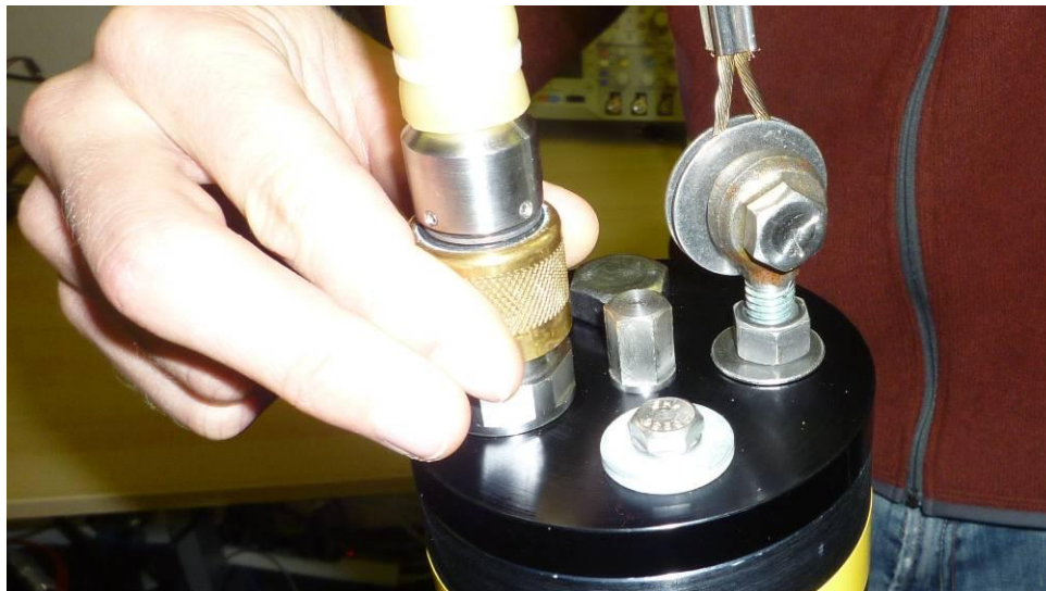
Figure 8: Connecting the MHDG cable (tether cable shown) on the VMP-200-RT rear bulkhead.
