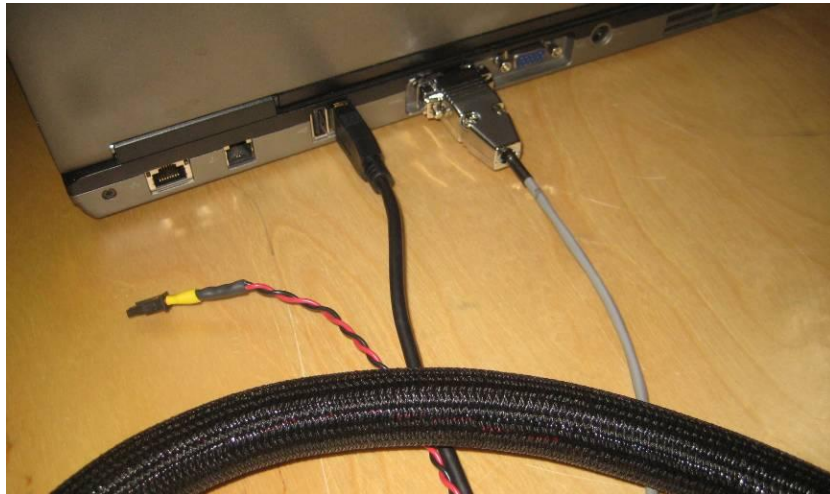
Figure 1: Connecting the deck cable to the computer.
