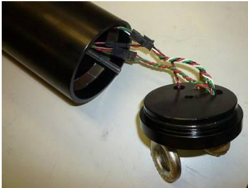
Figure 20: Rear bulkhead removed showing Molex Connectors.
