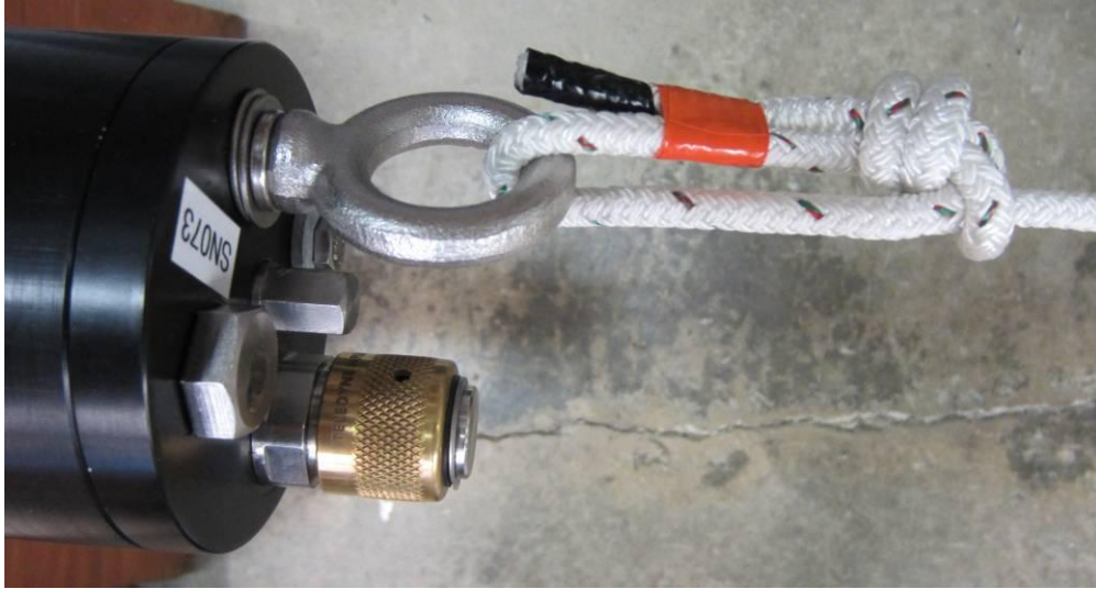
Figure 14: Attaching rope tether to VMP-200-IR.
