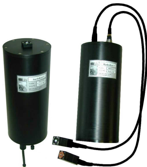
HydroRad-E1 with a plane irradiance collector and HydroRad-2 with one plane irradiance and one radiance collector.
