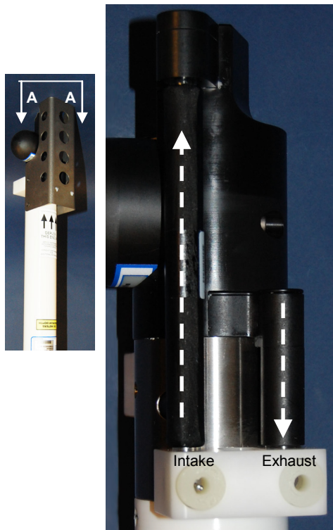
Shown with conductivity cell guard removed
