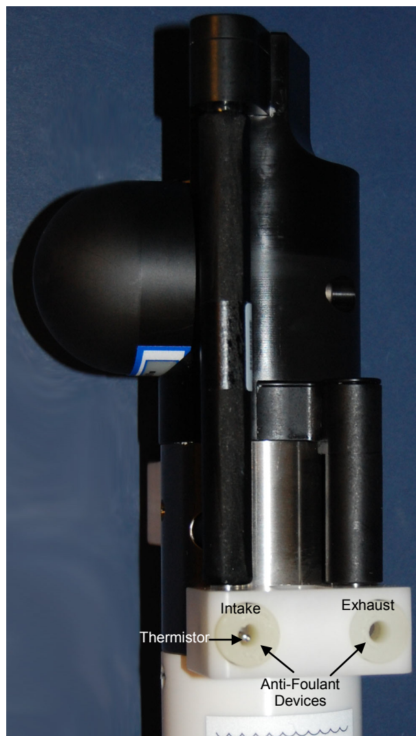
Shown with conductivity cell guard removed
