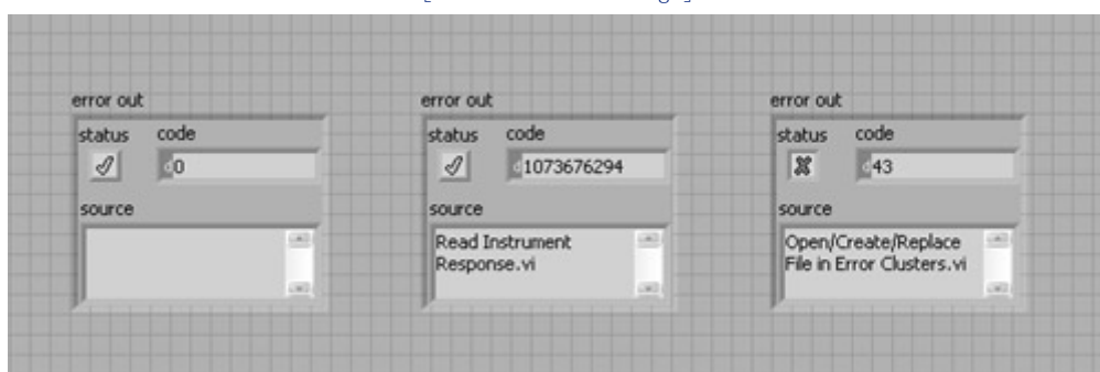
Figure 7-1. The error out clusters indicate no error or warning on the left, a warning in the middle, and an error on the right.
