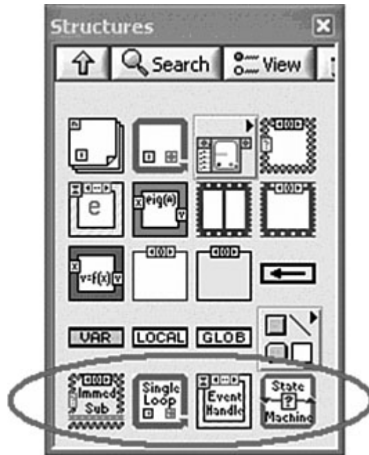
Figure 8-17A. Custom palette view contains several icons representing single-loop design patterns. The icons are configured to merge the corresponding design pattern onto the selected diagram.
