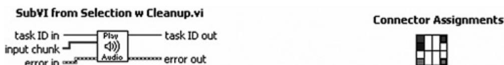
Figure 5-14B. SubVI from Selection w Cleanup VI contains a meaningful icon, intuitive terminal labels, and the standard 4x2x2x4 connector pattern.
