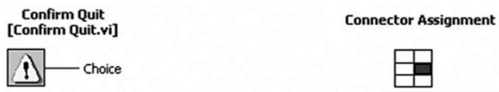
Figure 5-21B. The icon has been modified to indicate the type of confirmation. The standard 4x2x2x4 connector pattern has been applied, as well as the assignment of error terminals to facilitate execution ordering.
