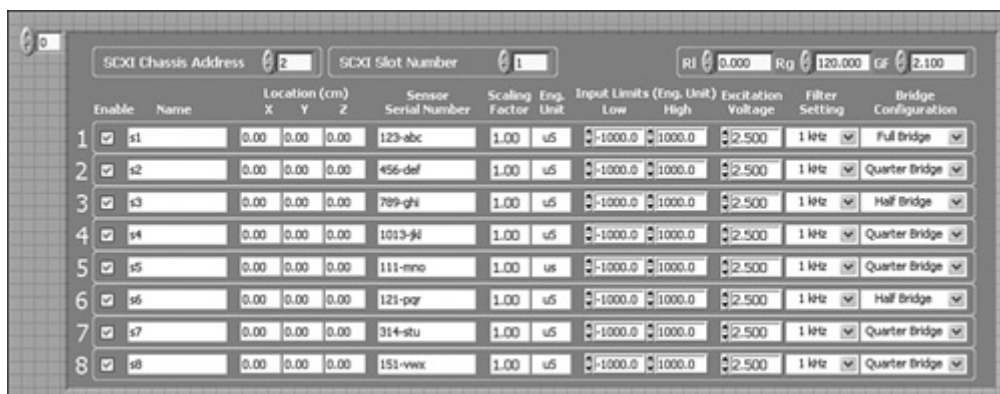
Figure 6-16B. This array of cluster containing strain gage configuration parameters is one of seven data structures used on the Configure tab to configure a corresponding SCXI module type. On the GUI VI panel, the array index control is not visible and the background is transparent.
