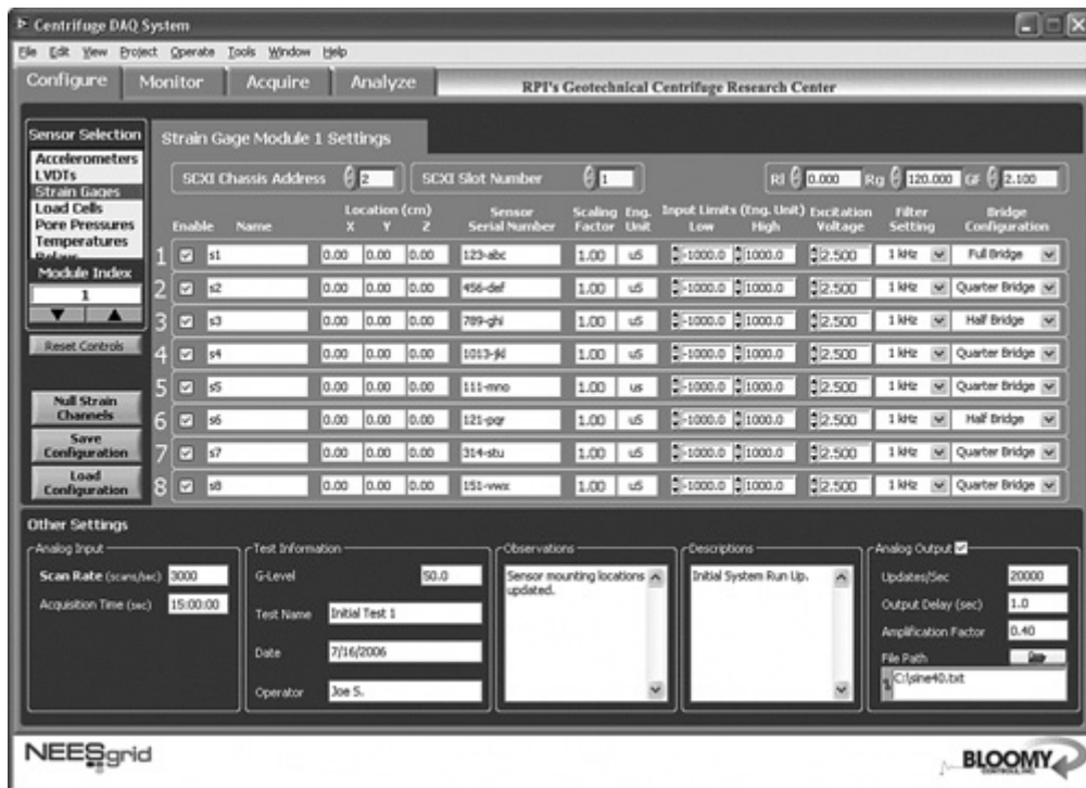
Figure 6-16A. The GUI VI panel for a highly configurable centrifuge data acquisition system [View full size image]
