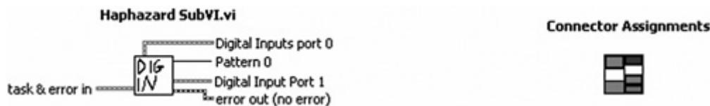
Figure 5-15B. The subVI icon has been improved using 8-point small fonts and a glyph of a pair of glasses. The DAQmx task passes through the top left and right terminals of the 4x2x2x4 connector pattern.
