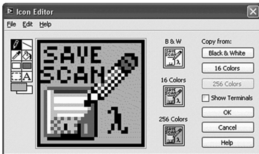
Figure 5-8. The floppy disk and pencil graphics are copied from an Express VI on the File I/O palette. The background color and text are customized, for distinction.
