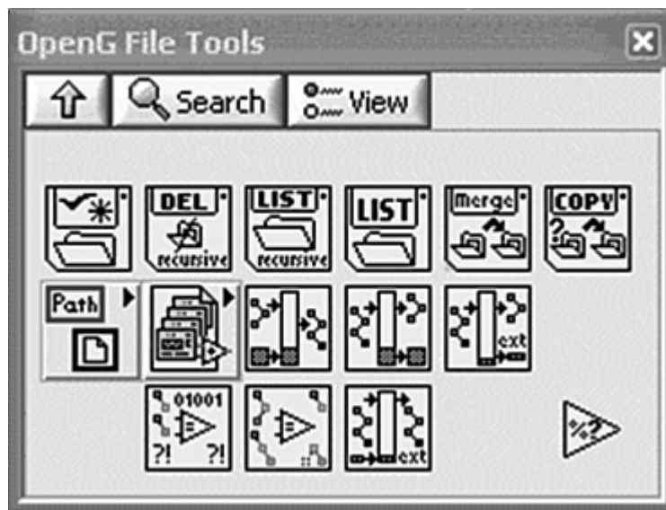
Figure 5-8. The floppy disk and pencil graphics are copied from an Express VI on the File I/O palette. The background color and text are customized, for distinction.
