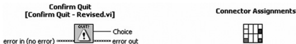
Figure 5-21B. The icon has been modified to indicate the type of confirmation. The standard 4x2x2x4 connector pattern has been applied, as well as the assignment of error terminals to facilitate execution ordering.
