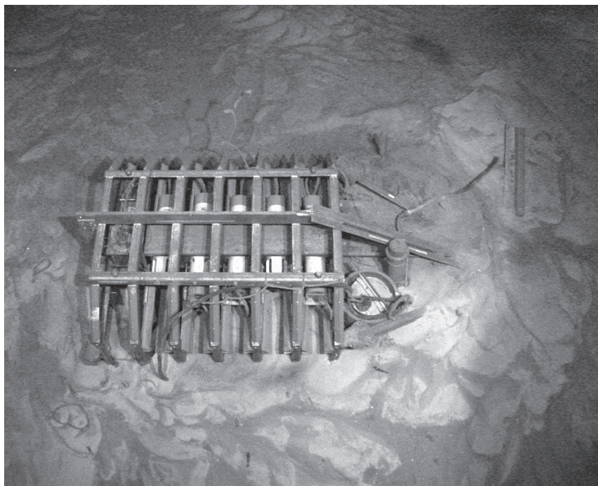
FIGURE 2-2 Seafloor junction box at HUGO, atop Loihi Volcano off Hawaii, after five years on the ocean floor. The partially buried package, recovered in October of 2002, is still in excellent condition. Use of titanium and plastics has virtually eliminated corrosion problems. Figure courtesy of Fred Duennebie, University of Hawaii.
