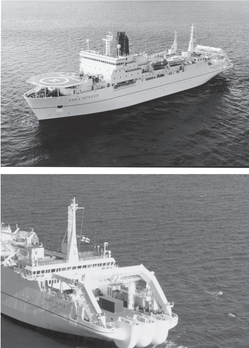
FIGURE 5-2 Photo of the Cable Retriever , a state-of-the-art, purpose-designed, all-stern working cable ship, equipped with an ROV (full view top; rear view bottom). This 117 m long vessel has a storage capacity of some 2,475 tons of cable. Specialized vessels such as this will be required for observatory cable installation and repair. Figure courtesy of Global Marine Systems Limited.
