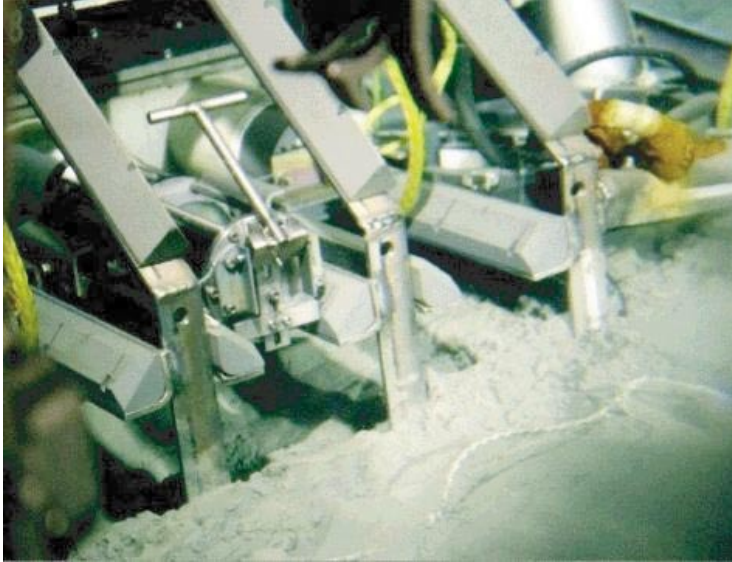
FIGURE 2-6 The starboard side of the HUGO junction box on Loihi seamount off Hawaii. Experiments are installed and repaired using the Pisces V submersible. SOURCE: Fred Duennebie, University of Hawaii.
