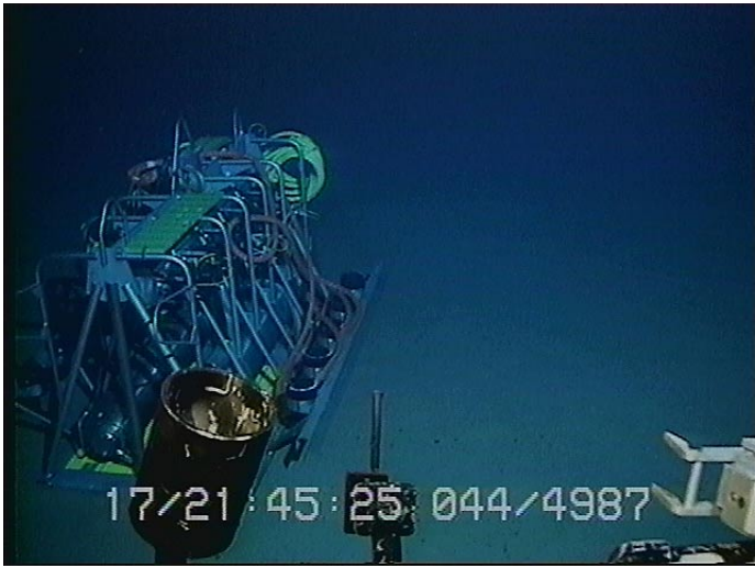
FIGURE 2-4 The Hawaii-2 (H2O) junction box on the seafloor as photographed by Jason. This junction box is designed to be removed for servicing and reinstalled by a research vessel and a remotely operated vehicle (ROV). SOURCE: Alan Chave, Woods Hole Oceanographic Institution.
