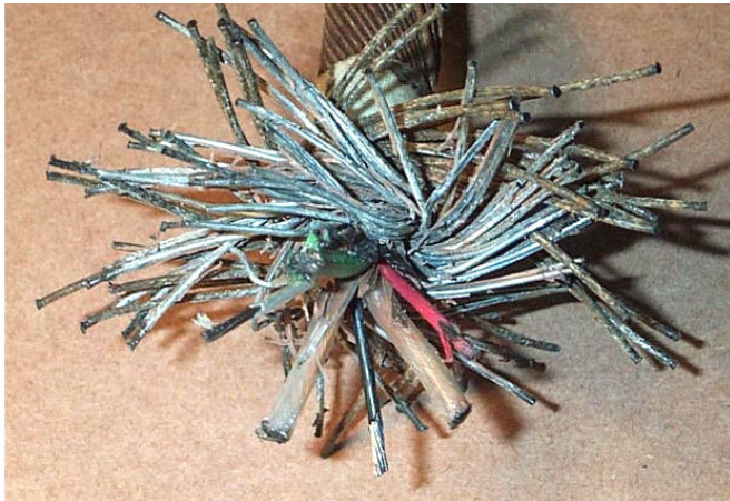
Fig. 2 Cable sample dissected for visual evaluation.
