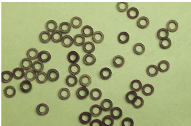
Fig. 3 Insulation sectioned and stained for voids, contaminants, and treeing inspection.
