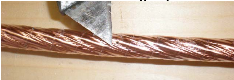
Failure Puncture in Copper Tape
