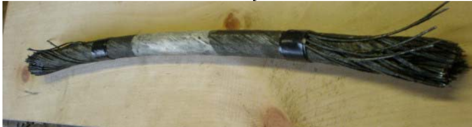
Cable Failure Ready for Dissection
