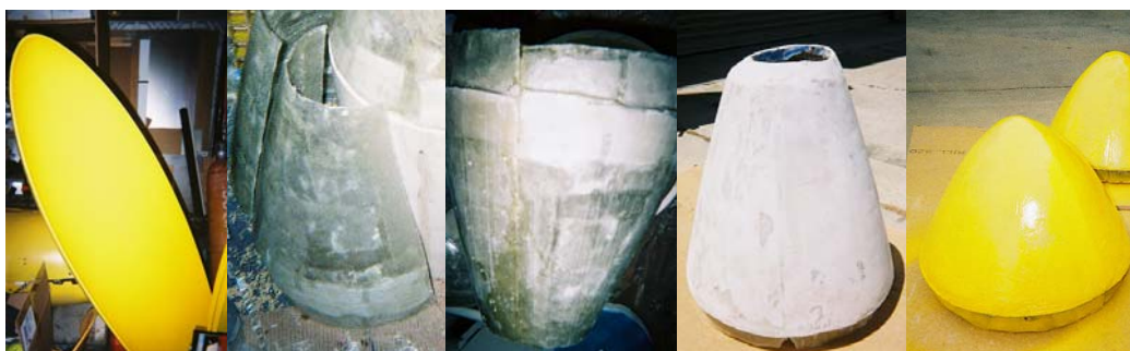
Figure 3.8 (a-e) Process used to create end caps from left to right: a) existing AUV shell used as a mold, b) end caps were created in halves, c) halves were joined, d) end caps were sanded and filled, and e) end caps were painted
