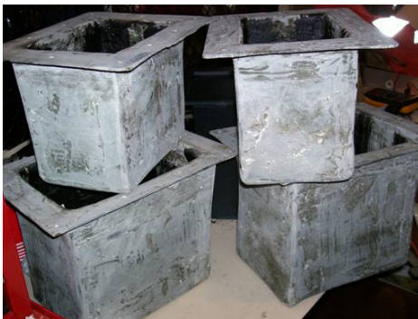
Figure 3.6. Fiberglass Resin Jelly Coat. Fiberglass resin jelly was used as another method to try and seal the fiberglass boxes. Unfortunately the boxes still had minor leaks.
