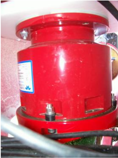
Figure 3.10 – Teledyne RDI Workhorse Doppler Velocity Log (DVL). This instrument uses sonar and the Doppler effect in order to provide high resolution velocity readings. It also has a high quality integrated attitude, heading, and reference system to provide heading, pitch, and roll data as well.
