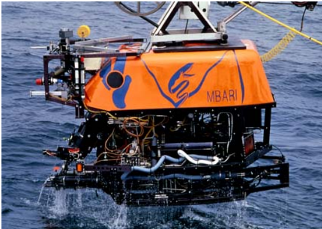
Figure 1.2 MBARI's Ventana ROV.[4]
