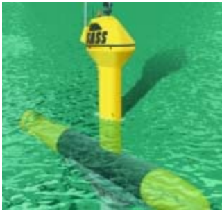
Figure 2.1 – ASV built by Autonomous Surface Vehicles Limited. This boat is powered by a diesel engine that can push it at a speed of ten knots while performing mapping.[12]
