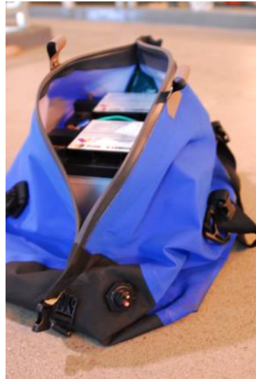
Figure 3.2 and Figure 3.3 – Previous Power Containment Devices. Sealed buckets (left), and sealed dive bags (right) have previously been used to enclose the batteries underwater and protect them from being flooded.
