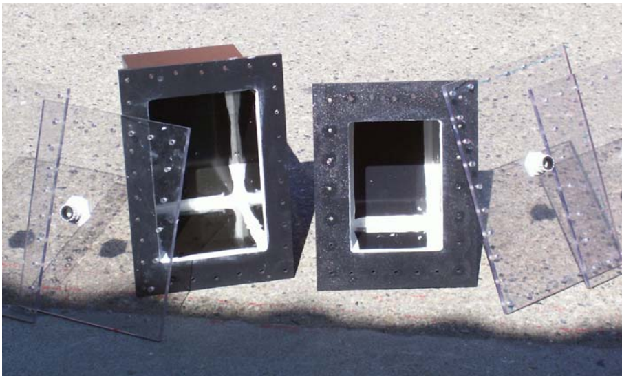
Figure 3.7 – Finished Waterproof ABS Battery Boxes. These boxes were assembled using 3/8 inch thick ABS plastic. The pieces were bonded using a solvent which melts the pieces together, creating a strong and watertight seal.
