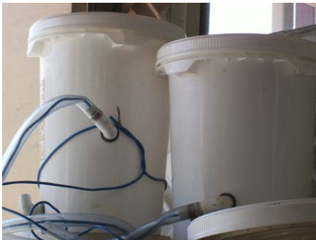
Figure 3.2 and Figure 3.3 – Previous Power Containment Devices. Sealed buckets (left), and sealed dive bags (right) have previously been used to enclose the batteries underwater and protect them from being flooded.
