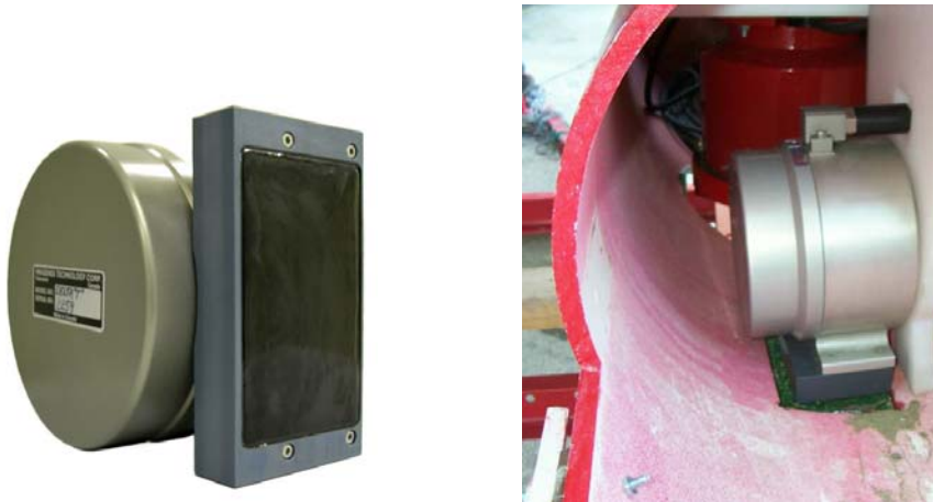
Figure 3.9 – Imagenex Multibeam Sonar. This multibeam unit is the primary instrument used to make maps. It emits 480 (300 KHz) sonar beams at an adjustable angle of up to 120 degrees. Left image is the manufacturer's image, and right image shows how it is mounted inside the hull.[9]
