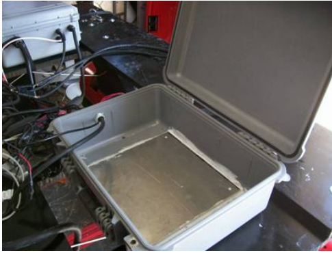
Figure 3.11 – Waterproof Laptop Enclosure. This Pelican case houses the laptop and prevents water from getting in. To remove some of the heat created by the laptop, the bottom of the box was replaced with an aluminum plate.
