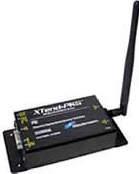
Figure 4.10: 9XTend-PKG-R™ 900 MHz RS-232/RS-485 RF Modem [19].
