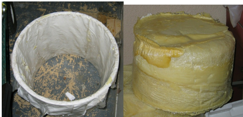
Figure 3.9 (a,b) a) Picture of the Mold for the Foam and b) a Foam Insert
