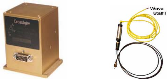
Figure 3. The Crossbow AHRS unit and the OSS Wave Staff II.
