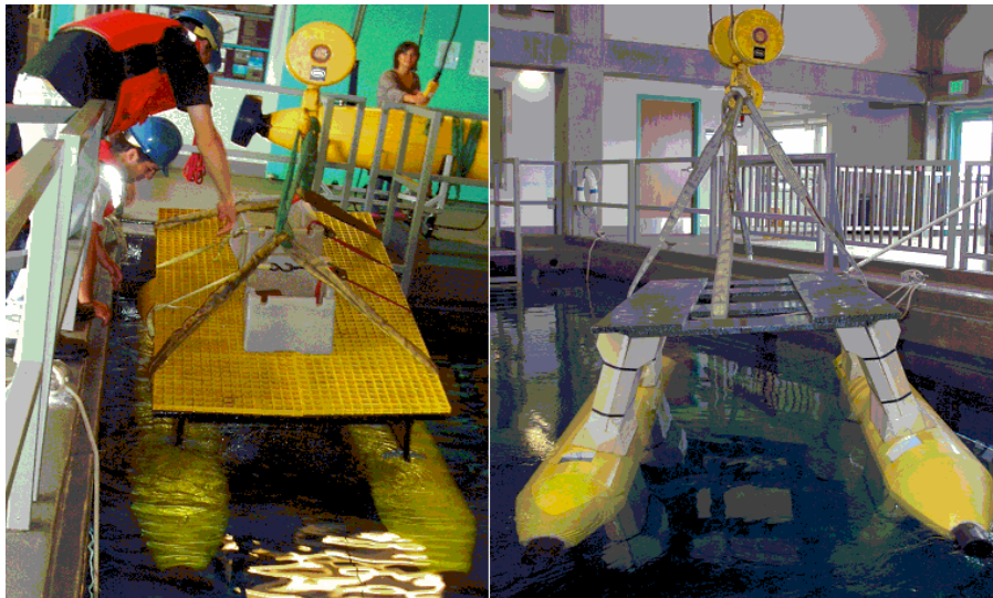
Figure 2. Shown to the left is the state at the beginning and to the right shows the top grating was removed to lower the CG, and 15^\circ wedges and the passive buoyancy packs were added.
