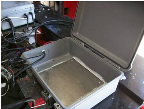
Figure 3.1 – Waterproof Laptop Enclosure. This Pelican case houses the laptop and prevents water from getting in. To remove some of the heat created by the laptop, the bottom of the box was replaced with an aluminum plate.
