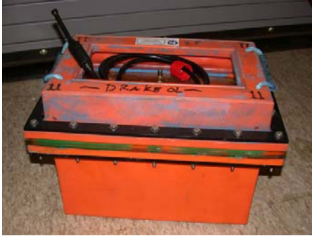
Figure 2.4 – Deep Ocean Engineering Waterproof Battery Enclosure. MBARI uses these sealed battery enclosures in their moorings.[6]
