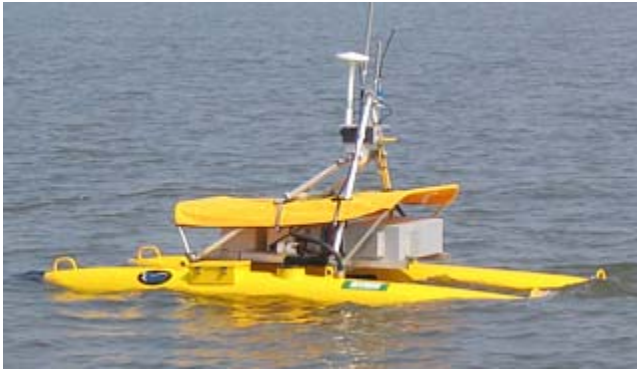
Figure 2.3 – USV-2600 by Sea Robotics Corporation. This ASV is equipped with a multibeam sonar and designed for shallow regions. It has been successfully deployed in the Florida panhandle[3].
