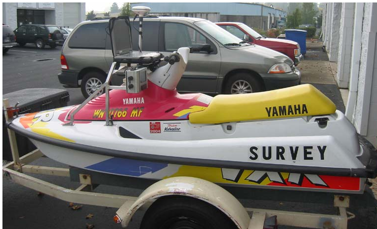
Figure 1.1 Seafloor Systems “Echo Runner”. This is a manned vessel equipped with an echo sounder to collect bathymetry data in shallow regions.
