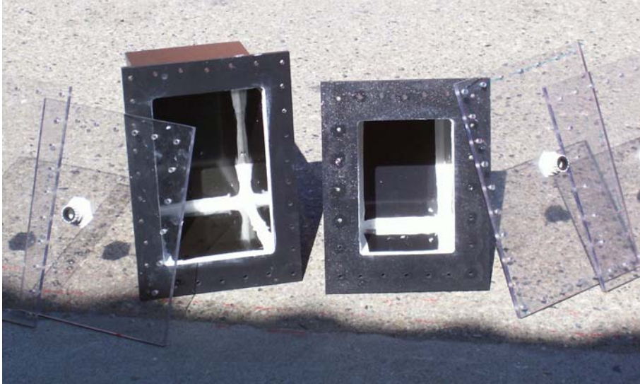
Figure 3.8 – Finished Waterproof ABS Battery Boxes. These boxes were assembled using 3/8 inch thick ABS plastic. The pieces were bonded using a solvent which melts the pieces together, creating a strong and watertight seal.
