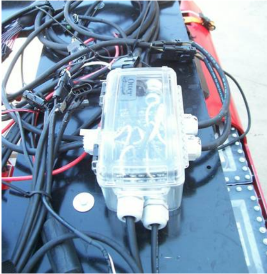
Figure 3.2 - Power Distribution Box. This waterproof box acts as a hub for the power system and provides 12 and 24 volts to the various subsystems.
