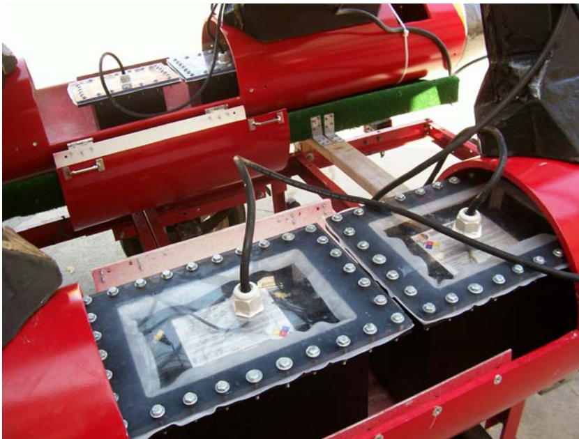
Figure 3.8 – Finished Waterproof ABS Battery Boxes. These boxes were assembled using 3/8 inch thick ABS plastic. The pieces were bonded using a solvent which melts the pieces together, creating a strong and watertight seal.
