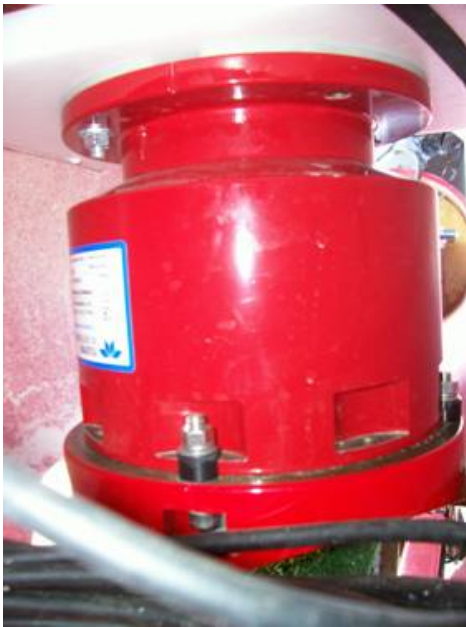
Figure 3.16 – Teledyne RDI Workhorse Doppler Velocity Log (DVL). This instrument uses sonar and the Doppler effect in order to provide high resolution velocity readings. It also has a high quality integrated attitude, heading, and reference system to provide heading, pitch, and roll data as well.
