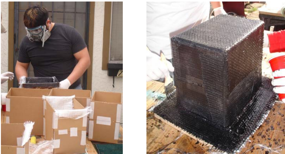
Figure 3.6. Fiberglass Construction Process. Cardboard frames were covered in fiberglass cloth and soaked in resin to create the rigid container.
