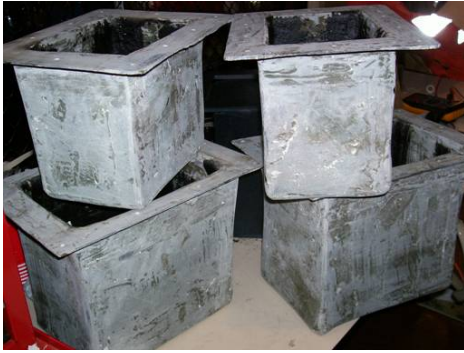
Figure 3.7. Fiberglass Resin Jelly Coat. Fiberglass resin jelly was used as another method to try and seal the fiberglass boxes. Unfortunately the boxes still had minor leaks.
