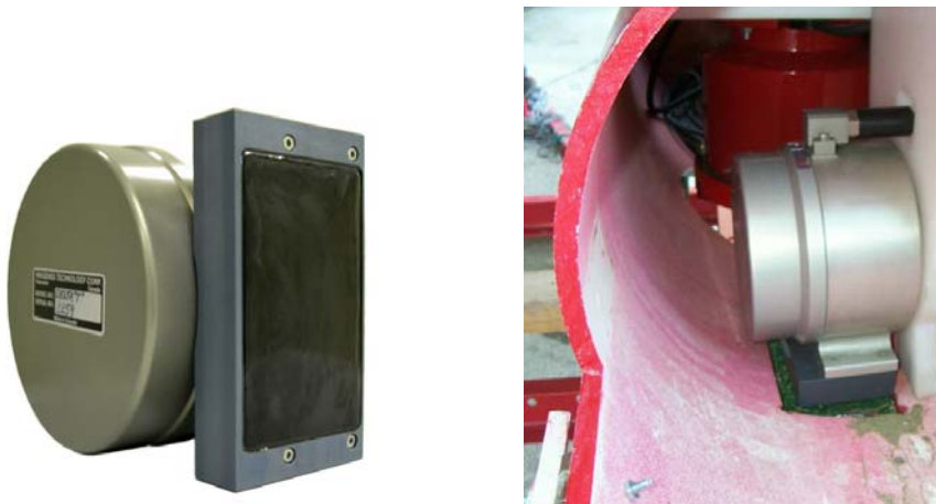
Figure 3.15 – Imagenex Multibeam Sonar. This multibeam unit is the primary instrument used to make maps. It emits 480 (300 KHz) sonar beams at an adjustable angle of up to 120 degrees. Left image is the manufacturer's image, and right image shows how it is mounted inside the hull.[9]
