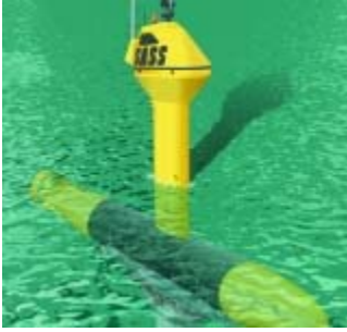
Figure 2.2 – ASV built by Autonomous Surface Vehicles Limited. This boat is powered by a diesel engine that can push it at a speed of ten knots while performing mapping.
