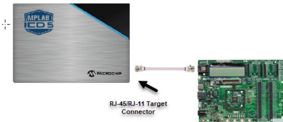
Figure 3-5. MPLAB ICD 5 Unit to Target Connection
