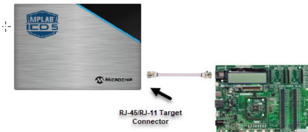
Figure 3-5. MPLAB ICD 5 Unit to Target Connection
