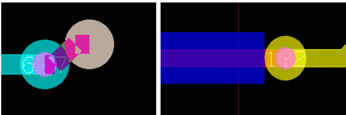
Figure 4-2 Via:Via =0 (left) and Via:SMD Pin=0 (right)
