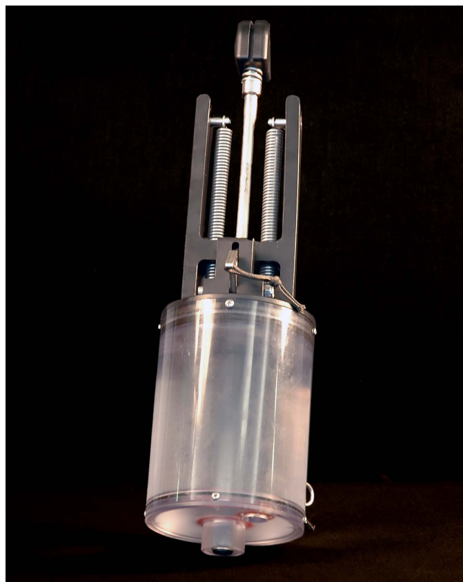
Figure 3. Rev 1.1 Prototype of Gulper sampler. Two extension springs drive the piston. The trigger cable passes over the head piece engaging the trigger. The sampler is open in unarmed position.
