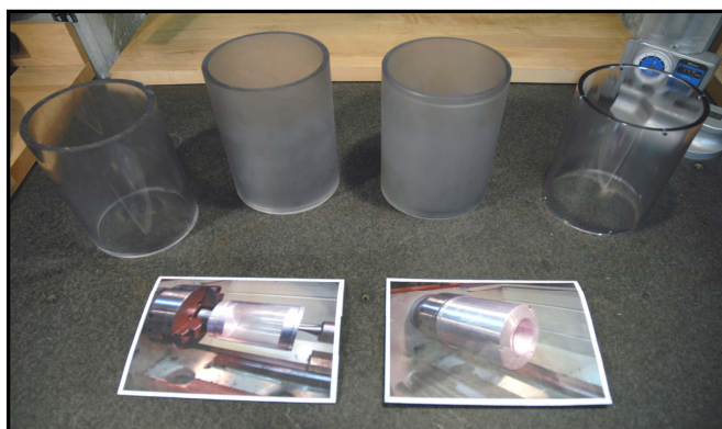
Figure 4. The Gulper sampler cylinders and dedicated tooling. Polycarbonate tubing has been machined and TCE vapor polished smooth and clear. The cylinders, from left to right, show the progressive stages in this process.
