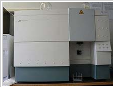
Front view of a desktop flow cytometer - the Becton-Dickinson Fluorescence activated cell sorter (FACSCalibur)
