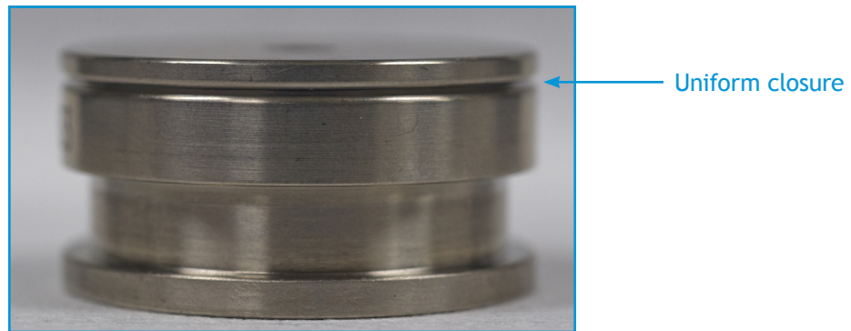
Figure 3-17: Uniform closure in properly assembled puck
