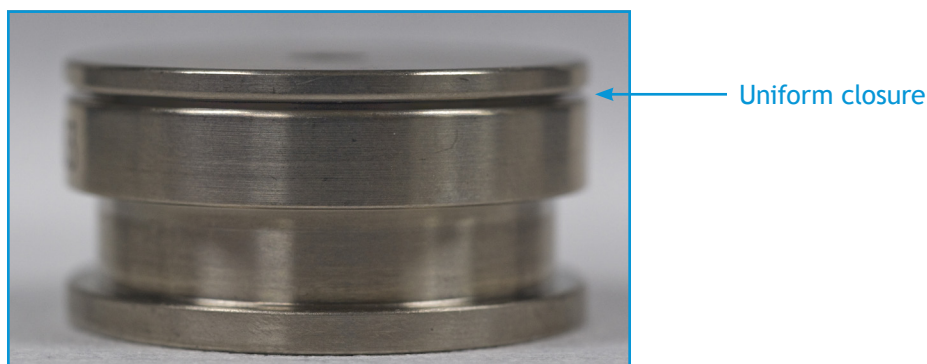
Figure 3-15: Uniform closure in properly assembled puck
