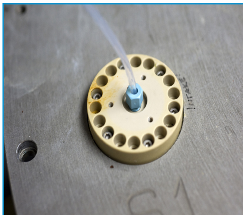
Figure 4-6: Sampling tube connected to Intake Port
