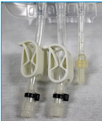
Figure 5-16: Male and female connectors on reagent bag
