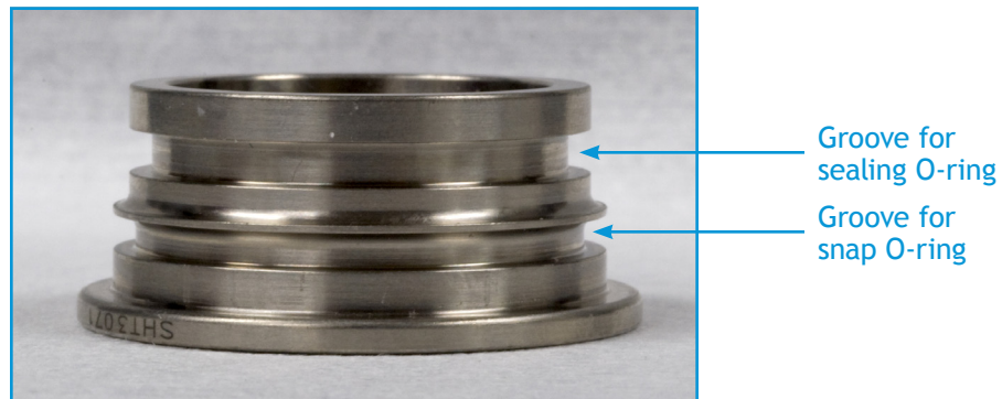
Figure 3-14: Close up of O-ring grooves in puck top
