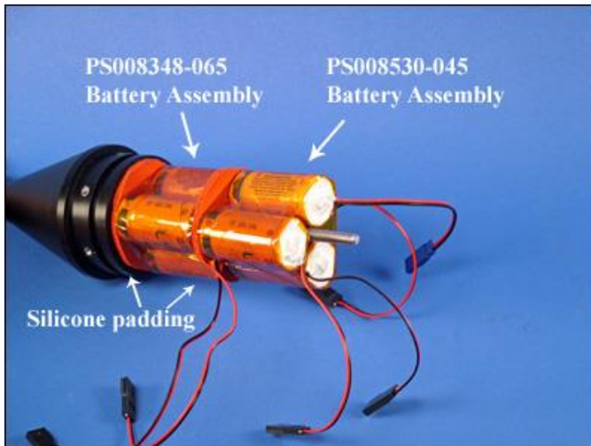
Fig. 6 Nose cone with both battery assemblies installed
