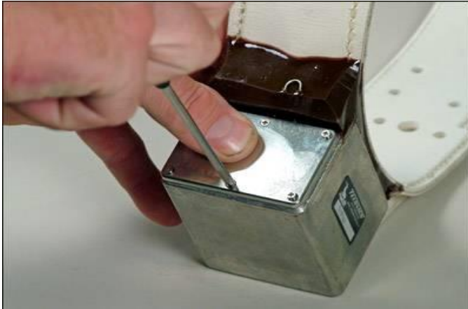
Fig. 1 Removing screws from TGW-4601
