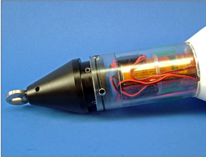
Fig. 9 VHF battery pack in nose cone cavity with nose cone ready to be inserted in housing.
