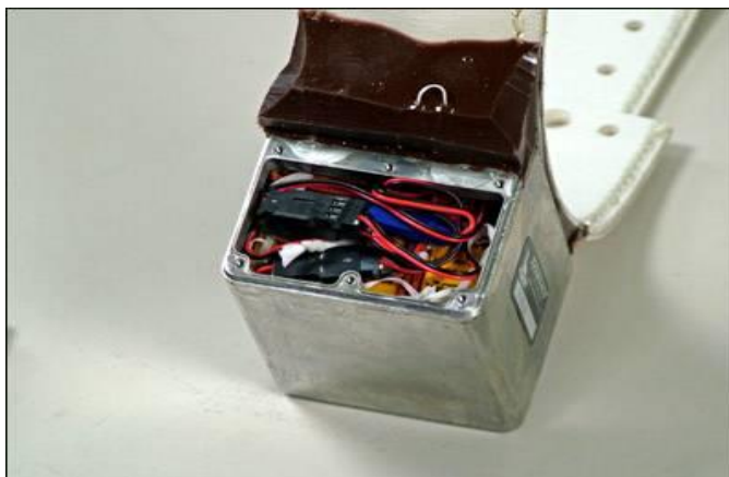
Fig. 4 All packs installed, Power leads folded down
