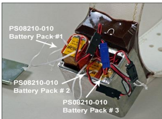
Fig. 2 Pack #1 ready to be removed from housing
