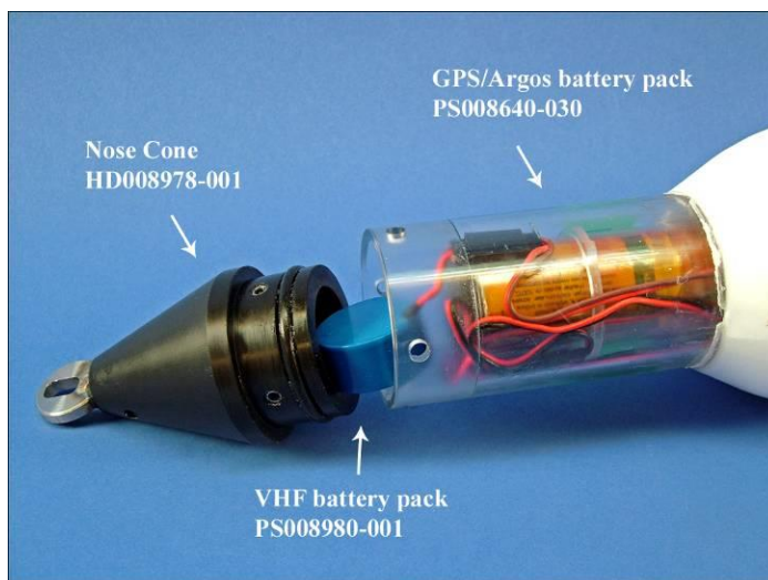
Fig. 8 VHF battery pack connected with connector properly placed between battery holder assembly and housing, ready to insert into nose cone cavity.
