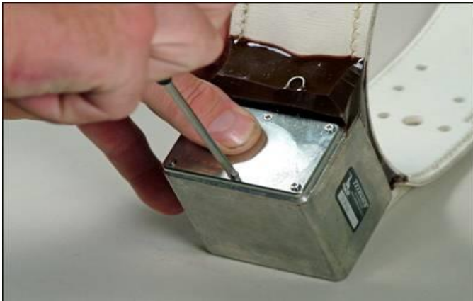
Fig. 6 Tightening screws, middle first
