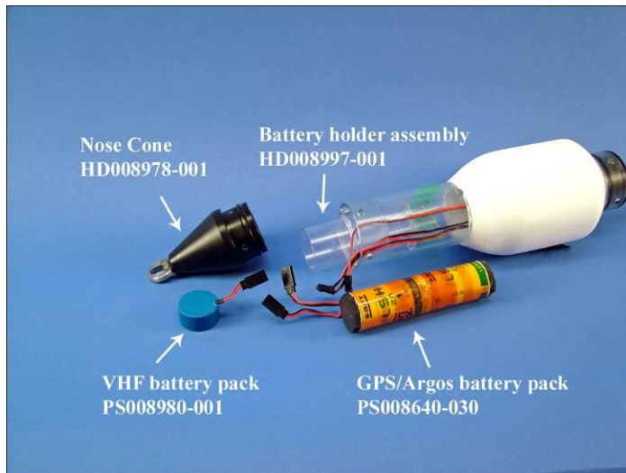
Fig. 3 Battery packs disconnected and removed from housing and nose cone showing GPS/ARGOS battery holder assembly protruding from the housing.
