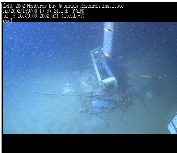
Figure 2. RIN after transport event buried frame in more than 70 cm of sediment and moved frame ~120 m down the canyon's axis (compare with figure 1). Empty battery case is bent around base of mast.
