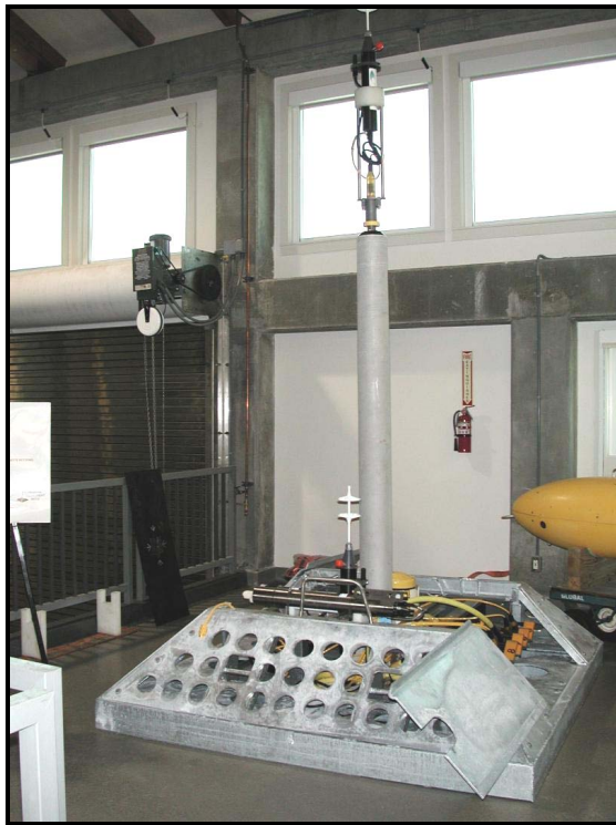
Figure 1. RIN platform outfitted with instruments before deployment (compare with figure 2).
