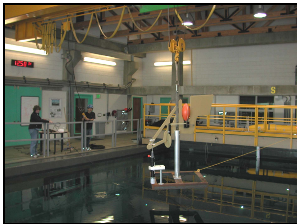
Figure 8. STED being lowered into MBARI Test Tank
