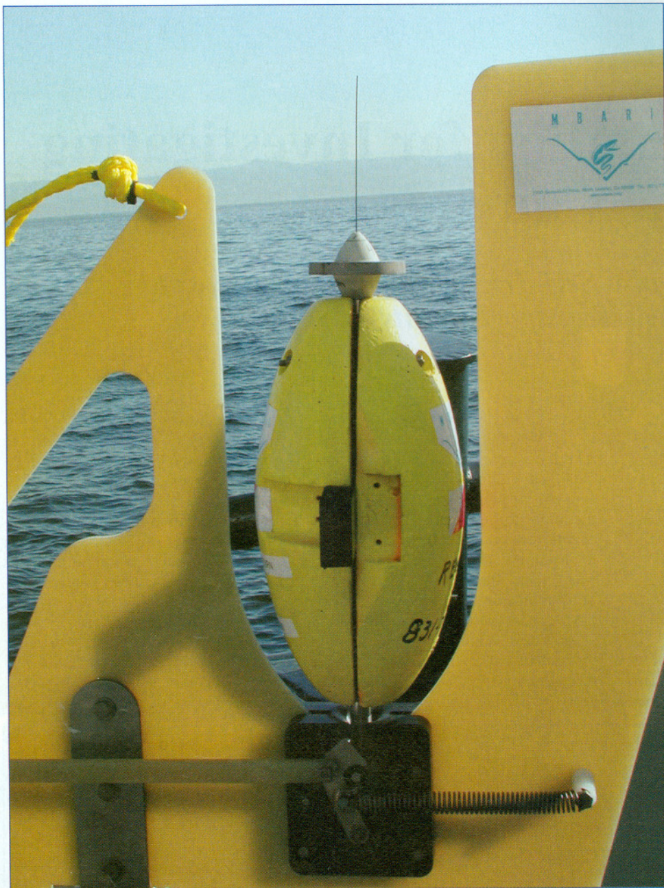
(Above) The vane section of a self-triggering event detector, including the mechanical release mechanism and science package with pop-up beacon.
